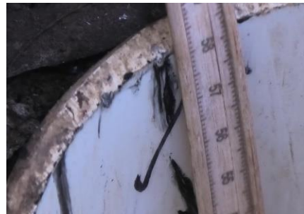
Use the measuring tape to read depth from top of the casing to the water level.
