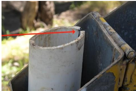
Always measure water levels from the same point on the casing.
